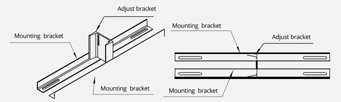
2) Install the assembled bracket on the conveyor frame with U-bolt.
