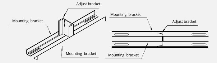
2) Install the assembled bracket on the conveyor frame with U-bolt.
